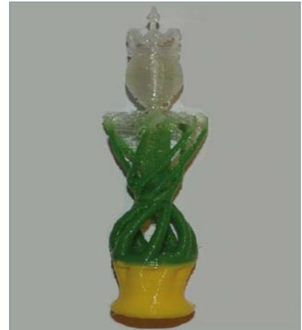
Figure 14. Model produced with three different filaments.
