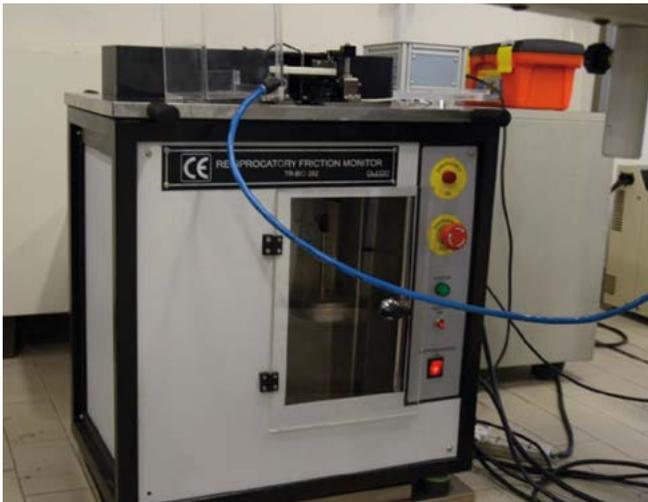
Figura 8. Tribómetro Reciprocatory Friction Monitor (DUCOM).
